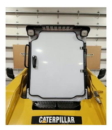
Step 15 – Your final inspection of your door installation should look as seen above, we recommend you follow the process suggested to ensure the desired result is achieved, once this has been done, you can loosen your secured points to peel the protective films for final and permanent install.
