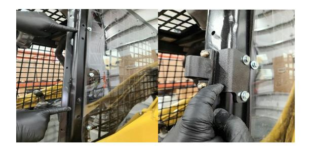
Step 9 & 10 – Locate these pre-existing side mount hole locations, attach your new hinge brackets as seen above, seat the brackets and let them rest on the bolts before securing, adjust accordingly for your best final fit.
