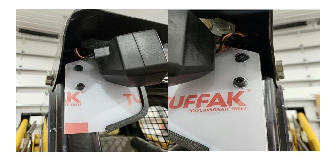
Step 5 & 6 Install and thread these holes with the supplied bolts and washers, tighten with a T40 Allen Key, be careful you don't overtighten and strip your threads.
