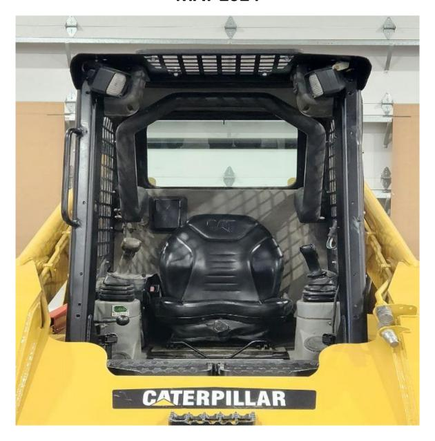
STEP 1) Remove ALL OEM equipment from your frame rails, you cannot use any previously existing hardware on your CAT A/B retrofit from SKID STEER DOORS of NORTH AMERICA.
