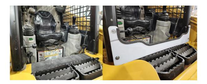
Step 7 & 8 – Locate these pre-existing hole locations, mount the bottom threshold with the supplied bolts, washers & locknuts, secure these using a 11 mm wrench and driver.
