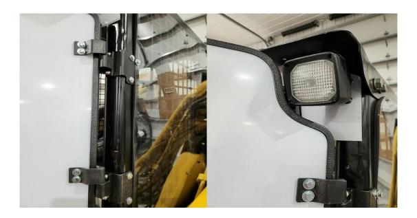
Step 11 & 12 – After mounting your male door hinge pins, drop the door onto the newly mounted side hinge brackets before adjusting your headlamp forward, if its done properly and there is no damage to your equipment, there will be no interferences with the door and your headlamps.
