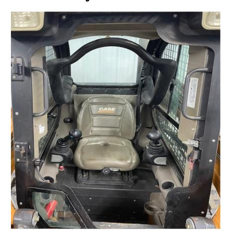
STEP 1) Remove ALL OEM equipment from your frame rails, you cannot use any previously existing hardware on your CASE SR / TR / TV retrofit from SKID STEER DOORS of NORTH AMERICA.
