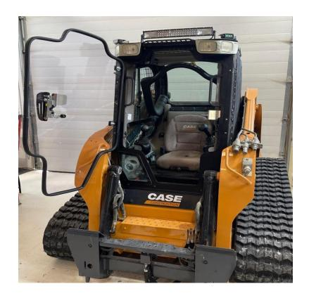
Step 12 – Your final inspection of your door installation should look as seen above, we recommend you follow the process suggested to ensure the desired result is achieved, once this has been done, you can loosen your secured points to peel the protective films for final and permanent installation.
