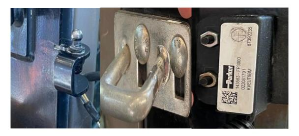
Step 2, 3 & 4 – Undo the air shock from the shock mount tower, locate your factory striker latch and remove. Locate and remove the magnetic door safety switch.
