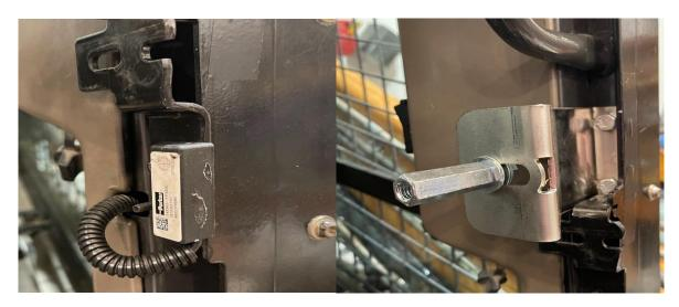
Step 9 & 10 – Re-install your magnetic safety door switch, rest your new Stainless Steel Z bracket ontop of your old striker mount, there mark your hole locations.
