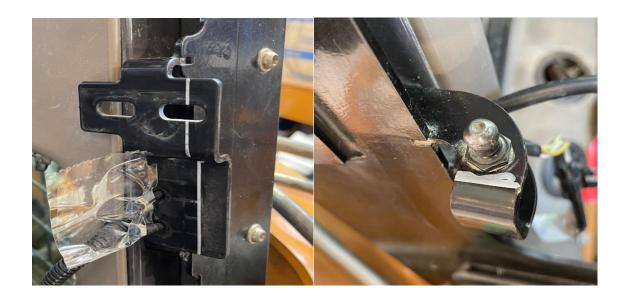
Step 5 & 6 – Locate your previous striker plate and shock tower mount, these locations will need to be trimmed back to allow for proper clearance of your new door which is flat, mark your trim line with a silver marker or paint pen, we recommend you cut this with a angle wheel grinder to get the best finish.
