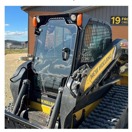
Step 12 – Your final inspection of your door installation should look as seen above, we recommend you follow the process suggested to ensure the desired result is achieved, once this has been done, you can loosen your secured points to peel the protective films for final and permanent installation.
