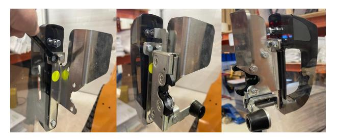
Step 11 – After mounting your door on the pre-existing factory male hinges, install your door handle, latch and stainless pull mechanism as depicted in images above, adjust as needed for best fit and acceptance of striker bolt.
